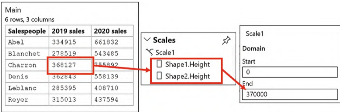
Figure 9-8. The Domain End value for “Scale1” is set by the field that is bound first
