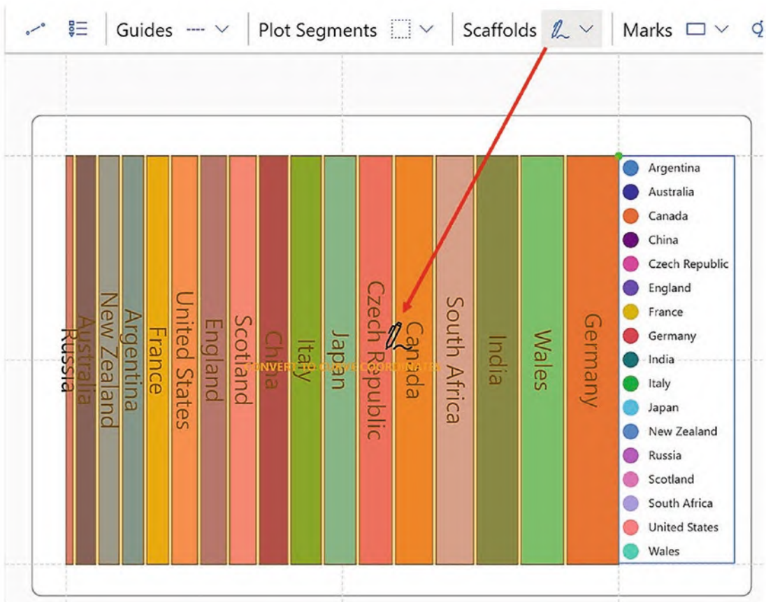
Figure 13-23. Applying a custom curve scaffold
